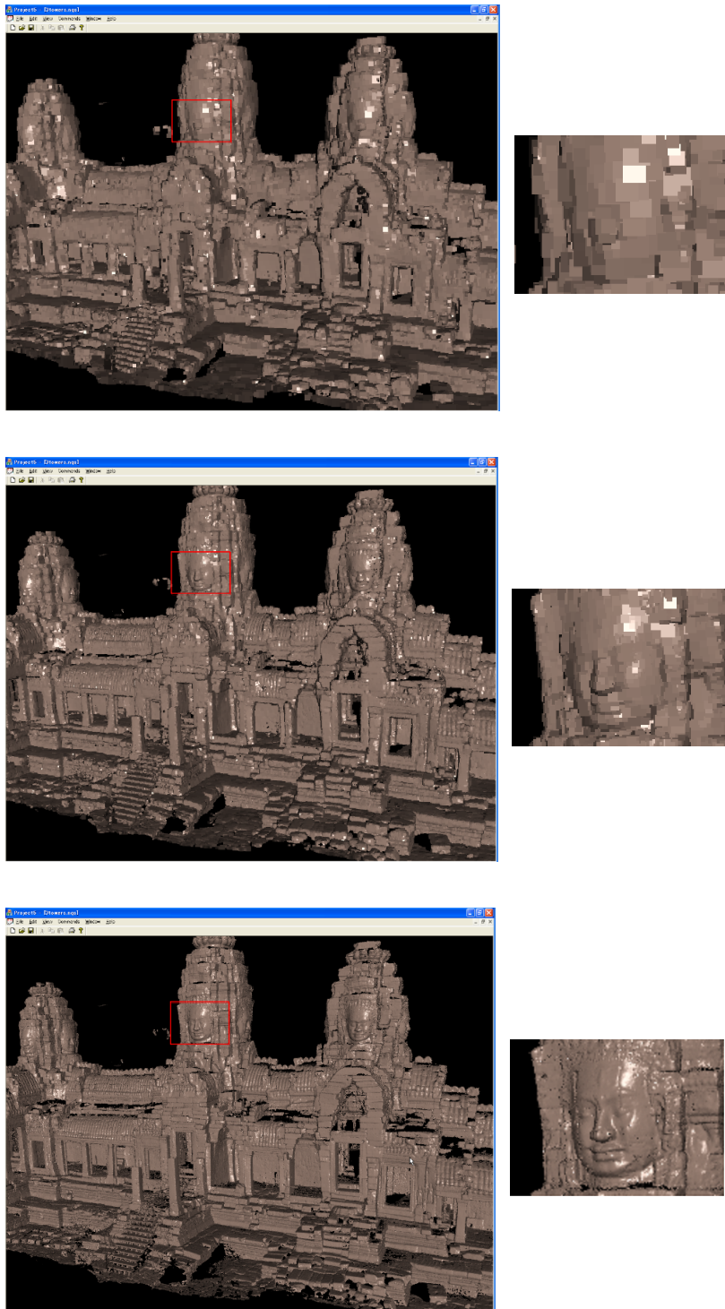
Figure 1.1: Multiresolution rendering : from top to bottom, the resolution increases. The images on the right are enlarged views.
