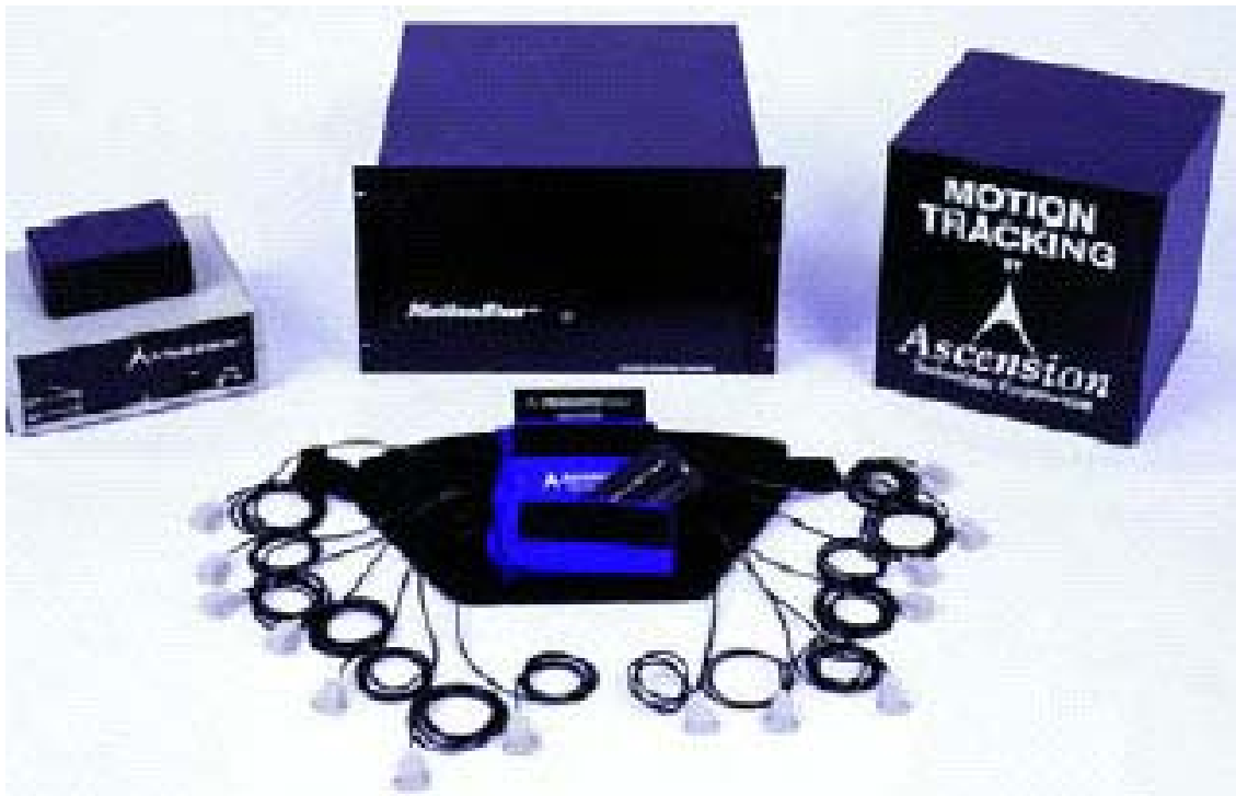
Figure 2.2 Magnetic type motion capture system; Ascension
