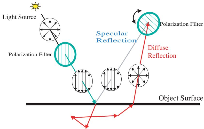
Figure 5.1: Mechanism of reflection components separation
