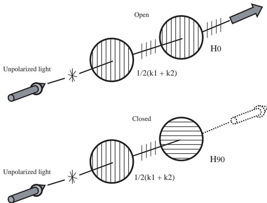
Figure 3.1: Transmissivity of a pair polarization filters
