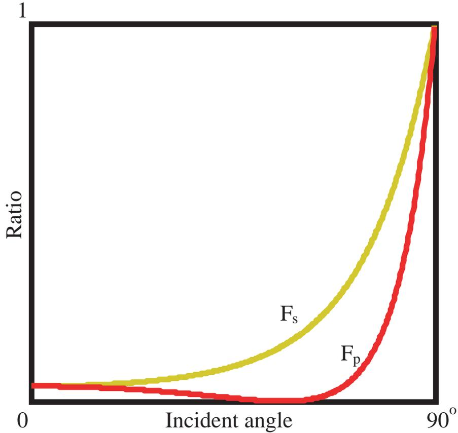
Figure 3.3: Relation between incident angle and Fresnel coefficients ( $F_p = F_{\parallel}, F_s = F_{\perp}$ )
