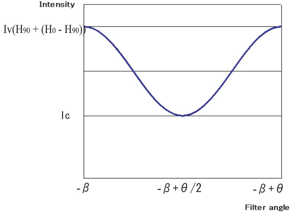
Figure 3.2: Relation between the image brightness and the orientation of a polarization filter
