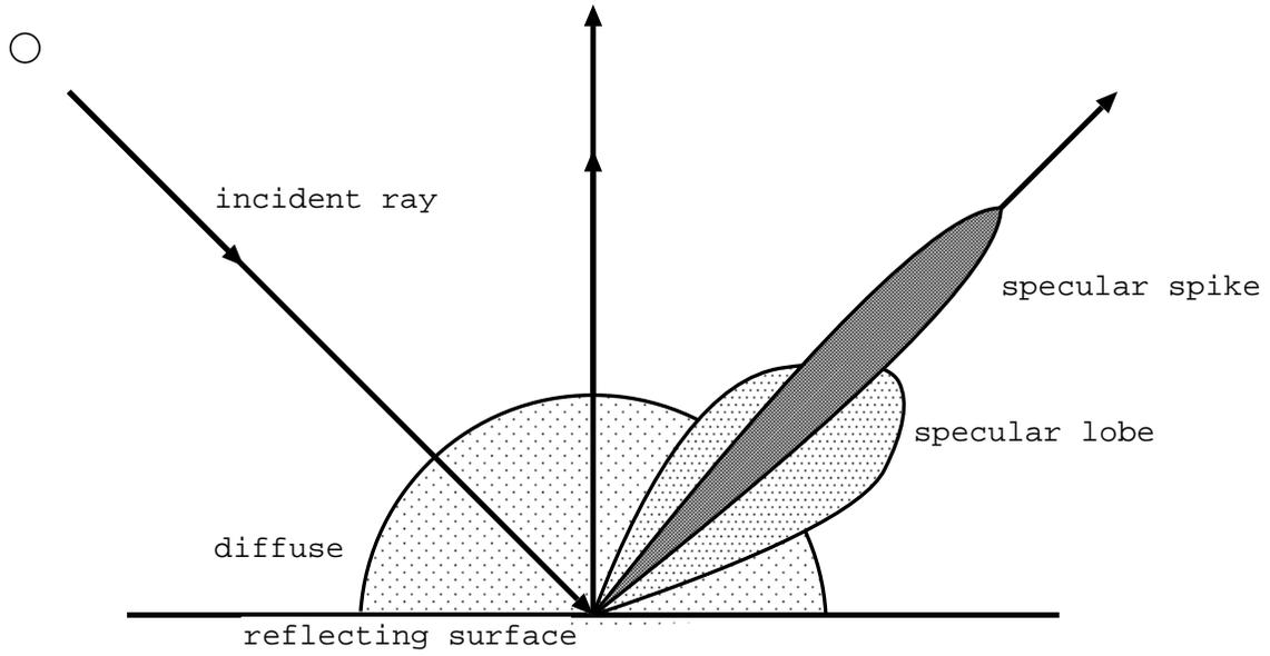
Figure 2.2: Diagram of the Unified Reflectance Model
