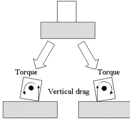
Figure 5.4: Torque in detaching a contact relations
