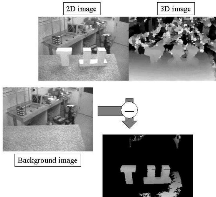
Figure 3.2: Extracting assembly parts using background subtraction
