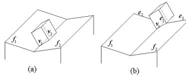
Figure 2.8: Parallel edge-edge contact
