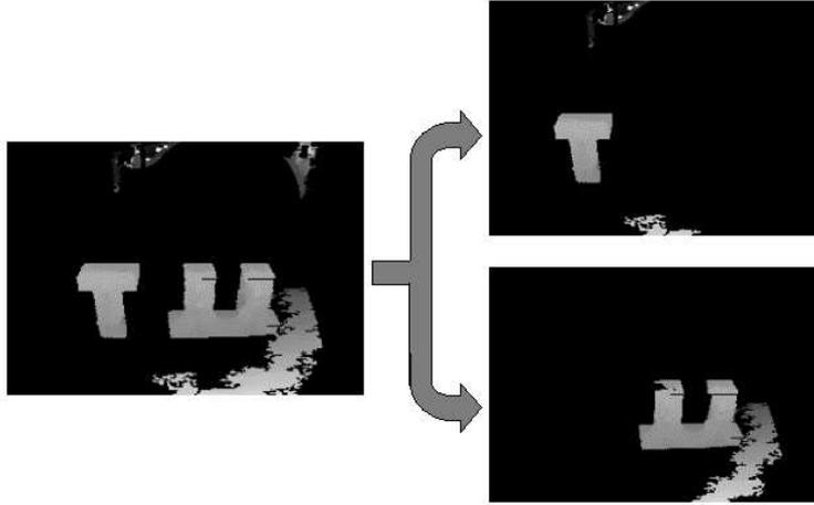
Figure 3.3: Dividing parts into a grasping and an environmental object
