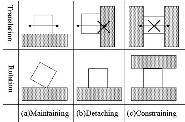
Figure 2.10: Three types of motion DOFs: maintaining, detaching, and constraining DOFs
