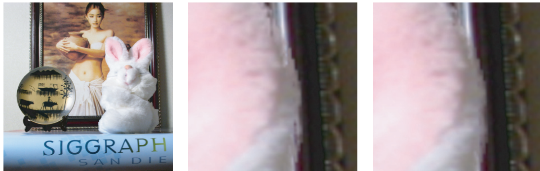
Figure 3.15: Comparison of results on a Furry rabbit, with video matting (middle image) and with coherence matting (right image). The alpha matte from coherent matting is smoother than that from video matting in the rendering image. This effect can be more clearly observed in the accompanying video.
