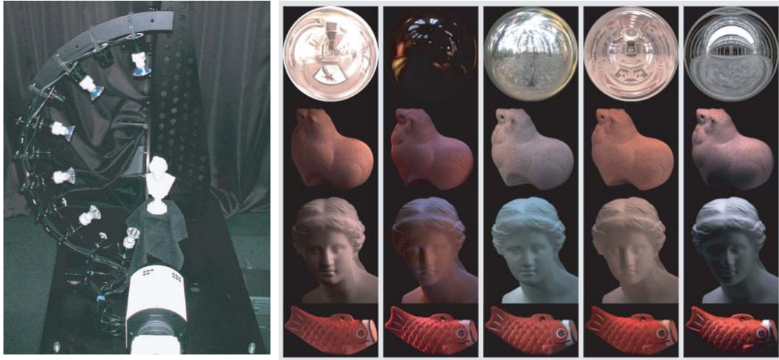
Figure 1.6: Hardware setup and synthesized images of objects under natural illumination. The first row shows illumination maps. The second, third and fourth rows show synthesized appearance of objects under the corresponding illumination map.
