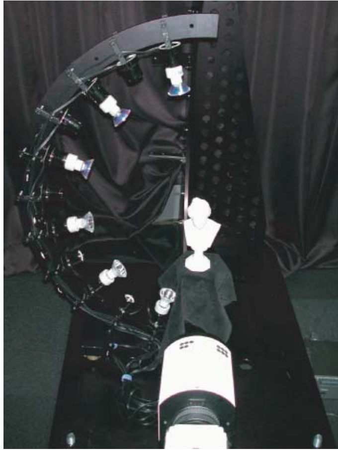
Figure 6.3: Image acquisition set-up: an array of light sources is mounted on a turntable. These light sources are equally spaced in elevation, and the set of light sources is rotated around the objects in azimuthal.
