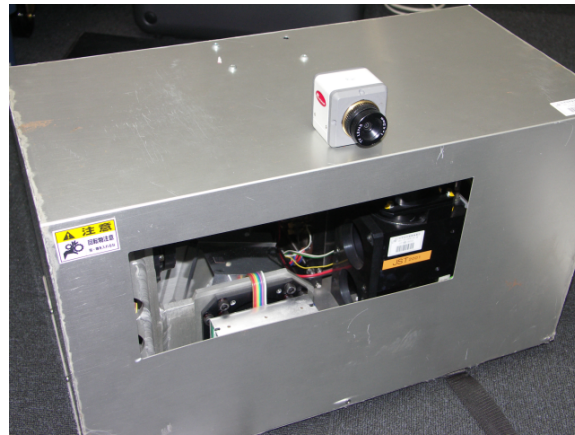
Figure 2.5: The monitoring camera mounted on the FLRS
