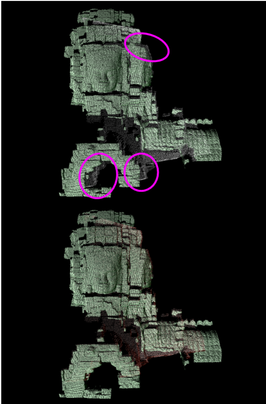
Figure 8.15: Range data before and after the rectification method without images: the upper figure shows the original distorted shape by the FLRS (white) and the reference shape obtained by the Cyrax-2500 fixed on the ground(blue). The lower figure shows the recovered shape in the lower figure (pink) fitted onto the correct one.
