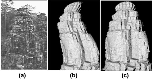
**Figure 2 Rectification of range image from the balloon sensor: (a) Scene, (b) distorted range image, (c) rectified range image using the Bannno-Ikeuchi**
