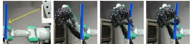
Fig. 4. Process of grasping: the position of a paintbrush is detected by the vision system (left), the hand approaches the paintbrush, and the power of the fingers is gradually added (right).
