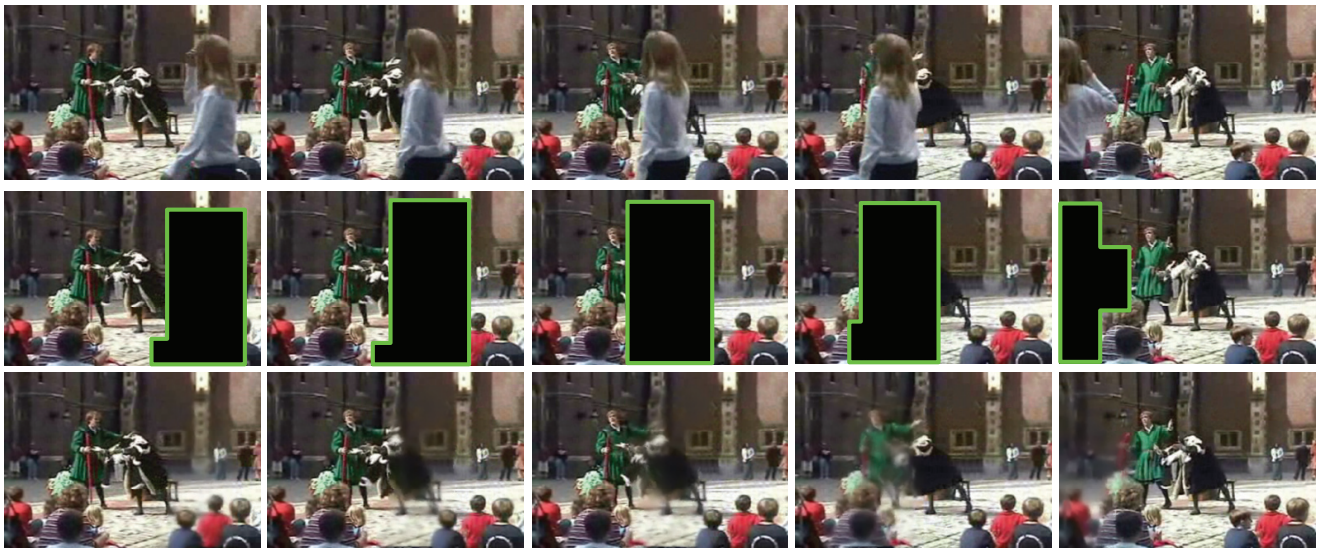
Figure 7. Object removal example (five representative frames shown). Top row: input video, where the two performers are occluded by a foreground person walking across the view. Middle row: after manually removing the foreground person. Bottom row: result of fill-in using our method.
