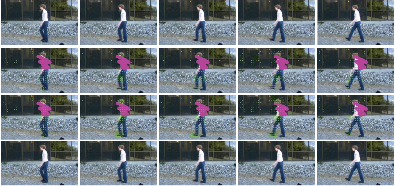
Figure 4. Walking scene result (five frames shown). Top row: original frames, second row: spatio-temporal hole and computed local motion field, third row: result of motion field transfer. bottom row: result of video completion. Notice the frames in the first and last rows are virtually identical.
