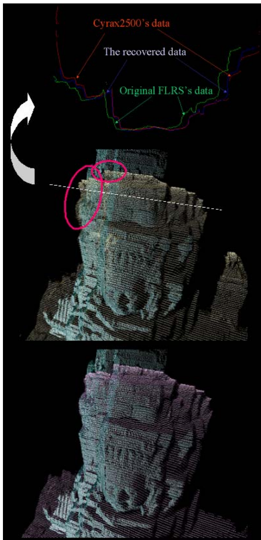
Fig. 3. Range data before and after the recovery process: The middle figure illustrates the registration of the original data from the FLRS (white) and the non-distorted data obtained by the fixed Cyrax 2500 (blue). Two shapes do not coincide, especially at the areas of ellipses in the figure. On the other hand, the recovered shape in the lower figure (pink) is fitted onto the correct data. The upper figure shows the cross section on the white dotted line in the middle figure.
