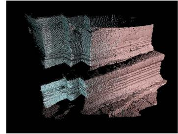
Fig. 8. The result of aligned range images: Red points represent the 3-D model obtained from a fixed sensor and light blue points represent the 3-D model obtained from the climbing sensor.
