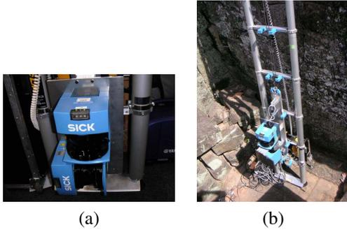
Fig. 1. (a) Two LMS200 scanners attached to our platform. (b) An overview of the climbing sensor.
