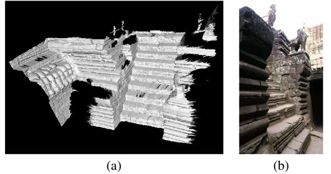
Fig. 7. (a) The result of the model obtained from the climbing sensor by placing the horizontal scan in an interval calculated from the vertical scan. (b) Actual scene of the target.
