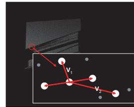
Fig. 5. Vectors to use for edge extraction.
