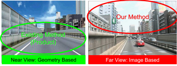
Fig. 3. Hybrid model expression: Near-view is represented by geometry-based model, and far-view is represented by image-based model.
