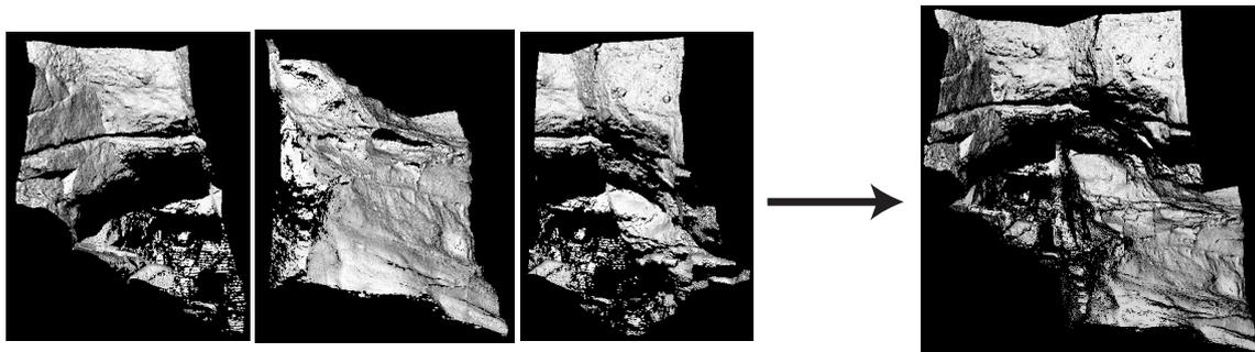
Figure 3: Alignment. Alignment can restore the relative position and posture between each corresponding pair of range images (left) as shown in the right illustration.
