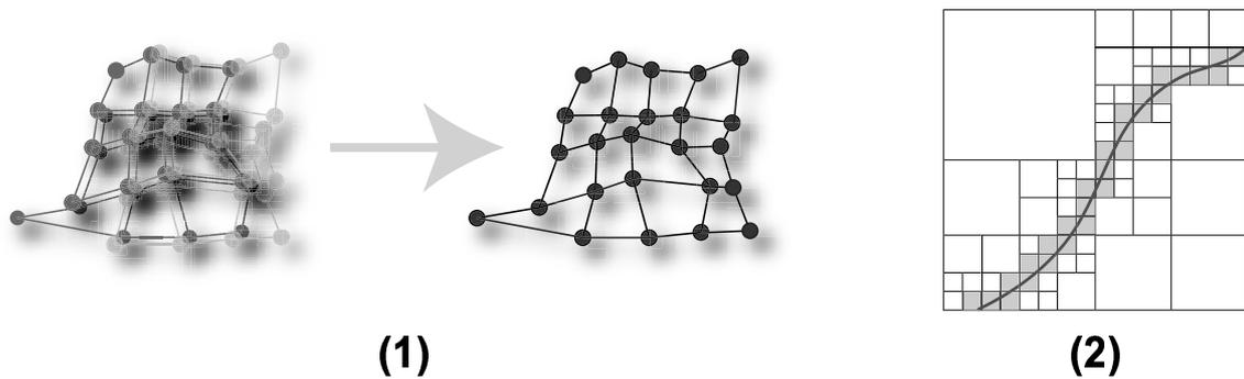
Figure 4: (1) Merging. Merging can integrate multiple aligned images (left side) into the single image (right side). (2) Voxel division by octree. Octree provides the effective merging because voxel division is adaptively performed only where the object surfaces exist.
