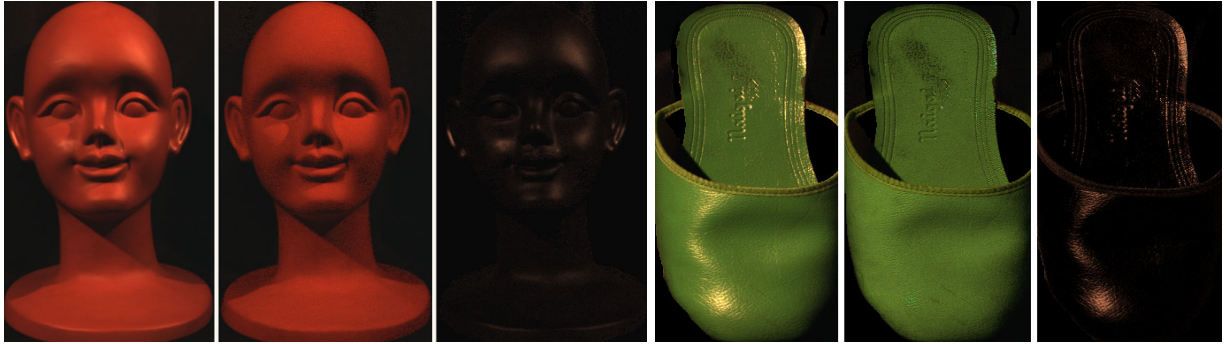
Figure 9: (a) Diffuse maximum chromaticity estimation for an image taken by SONY XC-55 (b) input image (c) diffuse reflection component (d) specular reflection component.
