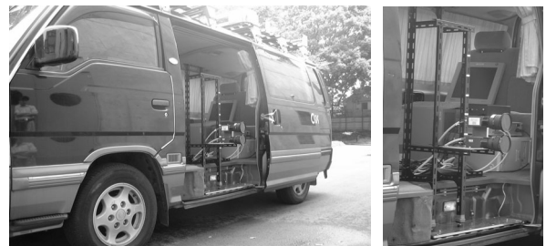
Fig. 5 Two line-scan cameras mounted on the measurement vehicle: a upper camera scanning vertically, and a lower camera scanning horizontally.
